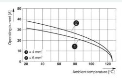
Derating diagram (6 modules in HC-B 24 housing)
