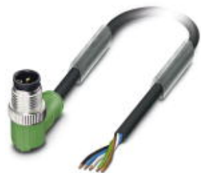
Sensor/actuator cable, 5-position, PUR halogen-free, black-gray RAL 7021, Plug angled M12, A-coded, on free cable end, cable length: 3 m
