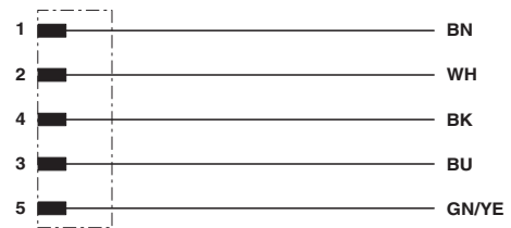
Contact assignment of the M12 plug
