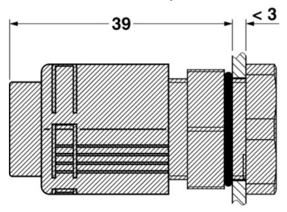
QUICKON panel feed-through with Q-SMU PG 13,5 safety nut, locked with Q-MU PG 13,5 counter nut.
