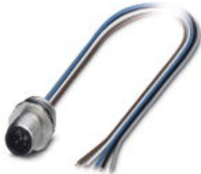
Sensor/Actuator flush-type plug, 5-pos., M12, A-coded, front/screw mounting with PG9 thread, with 0.5 m TPE litz wire, 5 x 0.34 mm 2
