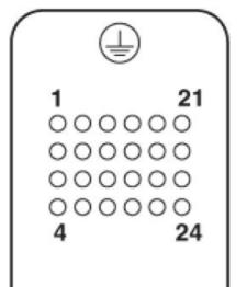
Connector pin assignment, connection side
