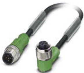
Sensor/actuator cable, 5-position, PUR halogen-free, black-gray RAL 7021, Plug straight M12, A-coded, on Socket angled M12, A-coded, cable length: 1.5 m
