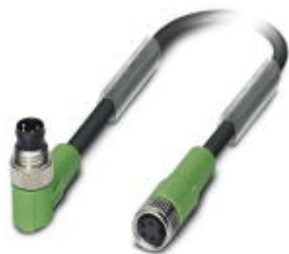
Sensor/Actuator cable, 4-position, PUR halogen-free, black-gray RAL 7021, Plug angled M8, on Socket straight M8, Cable length: 1.5 m
