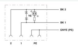
Contact assignment of the valve plug
