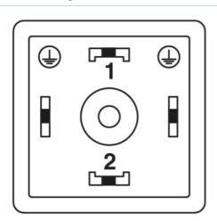
Valve connector pin assignment, type A
