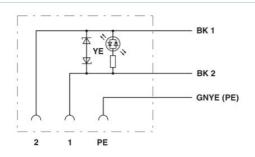
Contact assignment of the valve plug
