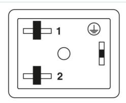
Valve connector pin assignment, type BI
