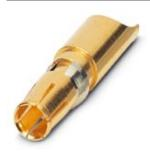
Power contacts, for D-SUB combination inserts, socket, solder cup, straight, rated current 40 A, gold-plated
