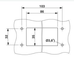
Panel cutout <sup>2</sup>) When self-tapping Torx screws are used (Torx20, M4)
