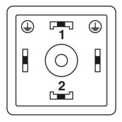
Valve connector pin assignment, type A
