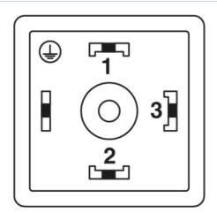
Valve plug connector pin assignment, type AD
