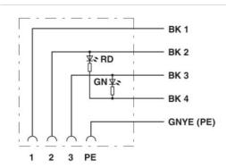
Contact assignment of valve connector
