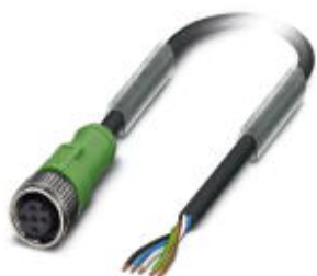
Sensor/actuator cable, 5-position, PUR halogen-free, black-gray RAL 7021, free cable end, on Socket straight M12, A-coded, cable length: 15 m
