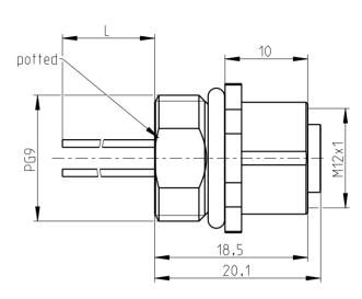
All specified data refers to the mounted M12 installation plugs  $\geq$  IP54 and requires abels or PCB mounting are also to be taken into consideration.
