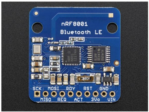
The nRF8001 is nice because it handles all the BLE radio and low level work, and does it all over SPI which makes it easy to use with any kind of microcontroller. All pins you need are broken out on the bottom of the PCB and all are 5V compliant so you can use with 3V or 5V micros!
