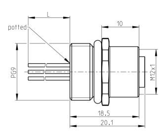
All specified data refers to the mounted M12 installation plugs ≥ IP54 and requires that the connector pair be correctly plugged and locked. Influences from wires, cables or PCB mounting are also to be taken into consideration.
