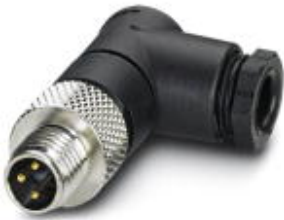
Connector, 3-position, Plug angled M8, A-coded, Solder connection, knurl material: Nickel-plated brass, external cable diameter 3.5 mm ... 5 mm
