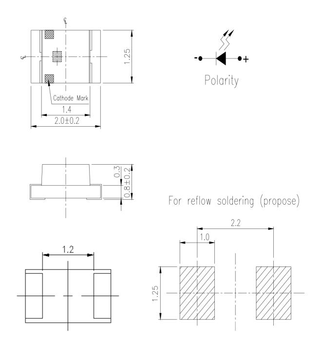
**Note:** The tolerances unless mentioned are  $\pm 0.1$  mm ,Unit = mm
