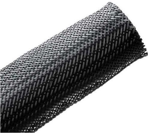
Braided Sleeve, Expandable, 1.25" Dia, PET, Black, 250 ft/bulk reel
