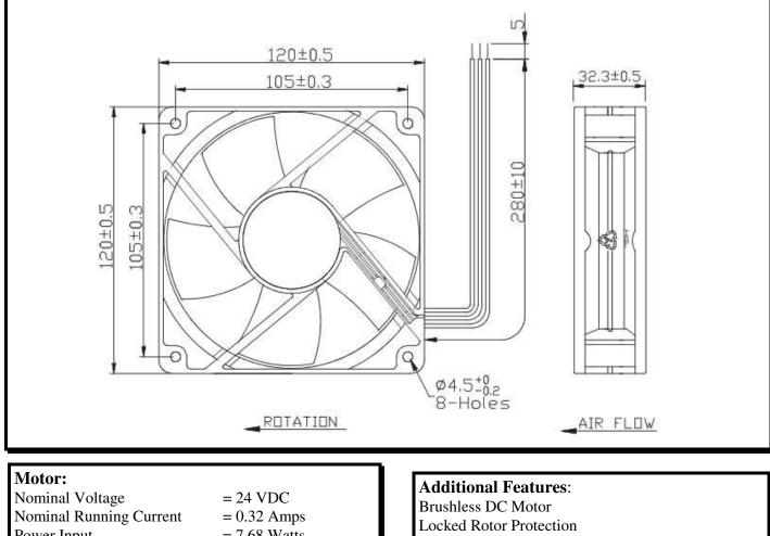
Power Input= 7.68Speed= 320Bearings= BalAir Flow= 133Static Pressure:= 0.32Acoustic= 48.4Weight= 213
