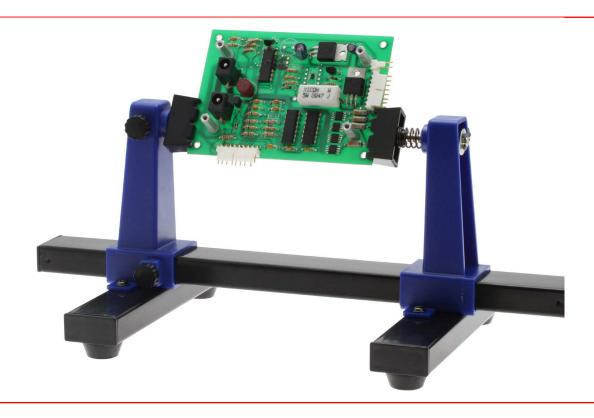
The Adjustable Circuit Board Holder is ideal for clamping PCB for soldering, desoldering or rework. It features 2 adjustable grips on a retractable stand to accomodate various board sizes up to 198mm wide and up to 4mm thick. The adjustable clamps allow the PCB to rotate 360 degrees and stay set in any position. The base of this rigid metal stand features four rubber feet to ensure stability.
