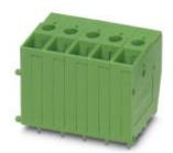
PC terminal block, Nominal current: 32 A, Nom. voltage: 630 V, Pitch: 7.62 mm, Number of positions: 1, Connection method: Screw connection, Mounting: Soldering, Conductor/PCB connection direction: 90 °, Color: green, The article can be aligned to create different nos. of positions!
