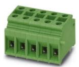
PC terminal block, Nominal current: 76 A, Nom. voltage: 630 V, Pitch: 10 mm, Number of positions: 1, Connection method: Screw connection, Mounting: Soldering, Conductor/PCB connection direction: 0 °, Color: green, The article can be aligned to create different nos. of positions!
