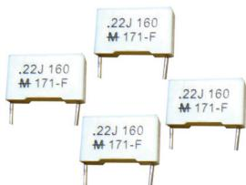
Type 171 radial leaded, box, metallized polypropylene capacitors are available in five pitch sizes and have a flame retardant case and epoxy encapsulant that meets UL94V-0. The Type 171 is an excellent choice for applications requiring low dielectric losses, high insulation resistance in an AC or DC environment. The polypropylene dielectric gives this capacitor excellent pulse rise time (dv/dt) performance.
