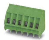
PCB terminal block, nominal current: 24 A, nom. voltage: 400 V, pitch: 5.08 mm, number of positions: 6, connection method: Screw connection with tension sleeve, mounting: Wave soldering, conductor/PCB connection direction: 55 °, color: green. The article can be aligned to create different nos. of positions!
