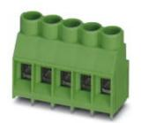
PCB terminal block, nominal current: 32 A, nom. voltage: 630 V, pitch: 6.35 mm, number of positions: 8, connection method: Screw connection with tension sleeve, mounting: Wave soldering, conductor/PCB connection direction: 0 °, color: green
