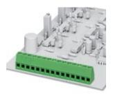
PCB terminal block, nominal current: 17.5 A, nom. voltage: 400 V, pitch: 5.08 mm, number of positions: 8, connection method: Screw connection with tension sleeve, mounting: Wave soldering, conductor/PCB connection direction: 0 °, color: green
