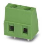
PC terminal block, Nominal current: 17.5 A, Nom. voltage: 630 V, Pitch: 7.5 mm, Number of positions: 2, Connection method: Screw connection, Mounting: Soldering, Conductor/PCB connection direction:  $0^{\circ}$ , Color: green, The article can be aligned to create different nos. of positions!
