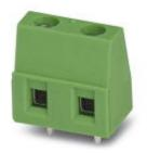
PC terminal block, Nominal current: 17.5 A, Nom. voltage: 630 V, Pitch: 7.62 mm, Number of positions: 2, Connection method: Screw connection, Mounting: Soldering, Conductor/PCB connection direction:  $0^{\circ}$ , Color: green, The article can be aligned to create different nos. of positions!
