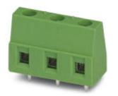
PC terminal block, Nominal current: 17.5 A, Nom. voltage: 630 V, Pitch: 7.62 mm, Number of positions: 3, Connection method: Screw connection, Mounting: Soldering, Conductor/PCB connection direction: 0 $^{\circ}$ , Color: green, The article can be aligned to create different nos. of positions!
