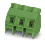
PC terminal block, Nominal current: 32 A, Nom. voltage: 1000 V, Pitch: 9.52 mm, Number of positions: 3, Connection method: Screw connection, Mounting: Soldering, Conductor/PCB connection direction: 35 °, Color: green, The article can be aligned to create different nos. of positions!
