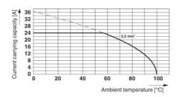
Derating diagram for 5 positions; reduction factor=0.8
