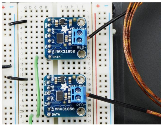
The MAX31850K data format is very similar to that of the well known 1-Wire DS18B20 temp sensor but it is *not drop in compatible* without code changes to check for the new '1 Wire family' type. We have adapted the classic Arduino <a href="OneWire">OneWire</a> (http://adafru.it/dal) and <a href="DallasTemp">DallasTemp</a> (http://adafru.it/dam) libraries to be MAX31850 compatible, so please click on those links to grab our libraries.
