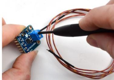
Insert the thermocouple wires and tighten down the clamps with a small Phillips or flat screwdriver
