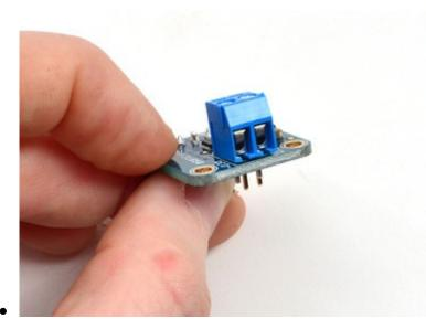
Now you can do the terminal block, this is what you'll use to attach the thermocouple since you cannot solder to thermocouples
