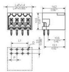
1728010000 S2L 3.5/10/90G 3.5SN SW PCB plug-in connector, Male connectors, Soldered connection, Pitch: 3.50 mm, No. of poles: 10, 90°, Box 4032248039500 50 pc(s).
