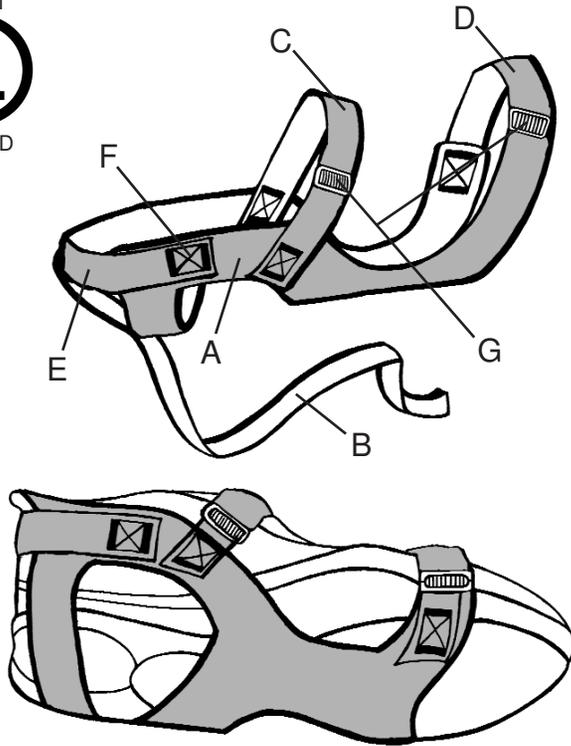
"For standing operations, personnel shall be grounded via a wrist strap system or by a flooring/footwear system. When a flooring-footwear system is used, one of the two following conditions shall be met:
