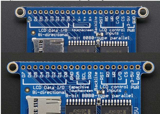
Make sure you're soldering and connecting to the 8-bit side!
