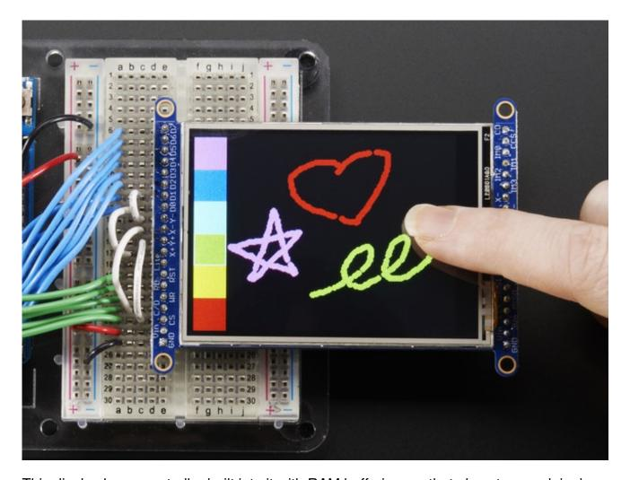
This display has a controller built into it with RAM buffering, so that almost no work is done by the microcontroller. **The display can be used in two modes: 8-bit or SPI.** For 8-bit mode, you'll need 8 digital data lines and 4 or 5 digital control lines to read and write to the display (12 lines total). SPI mode requires only 5 pins total (SPI data in, data out, clock, select, and d/c) but is slower than 8-bit mode.
