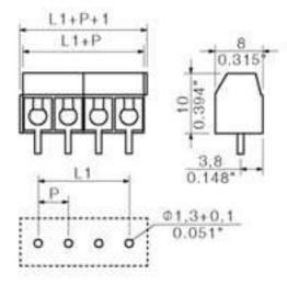
1760490000 PM 5.08/2/90 3.5 OR PCB terminal, Leaf spring connection, Soldered connection, Clamping range, max.: 2.5 mm<sup>2</sup>, Pitch: 5.08 mm, No. of poles: 2, 90°, Box 4032248032464 500 pc(s).
