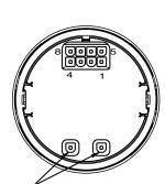
USED FOR DEVICE CONFIGURATION DO NOT CONNECT WHEN INSTALLING GAGE
