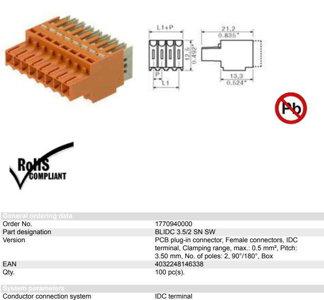
Outgoing direction of conductor Pitch Pitch in inch No. of poles No. of rows Screwdriver blade Screwdriver blade standard L1 in mm L1 in inch Electric shock protection to DIN VDE 0470 Electric shock protection to DIN VDE 0470 IDC terminal 90°/180° 3.5 mm 0.138 inch 2 1 0.4 x 2.5 DIN 5264-A 3.5 mm 0.138 inch IP 20 Safe from finger touch
