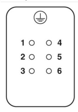
Connector pin assignment, connection side
