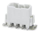
Header, Nominal current: 6 A, Rated voltage (III/2): 160 V, Number of positions: 3, Pitch: 2.5 mm, Color: white, Contact surface: Tin, Mounting: Taped SMD/THT/THR components
