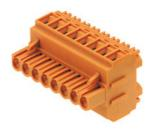
Female connectors with two clamping yoke screw connections per pole for conductor connection with 90° & 270° outlet direction. The female connectors provide space for labelling and can be coded. Packed in cardboard box.
