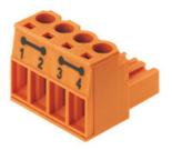
Female connectors with clamping yoke screw connection for conductor connection with straight outlet direction and internal cross-connection for connections 1-2 & Damp; 3-4. Bus current up to 32 A for 4 mm² (without wire end ferrules). The female connectors provide space for labelling and can be coded. Packed in cardboard box.
