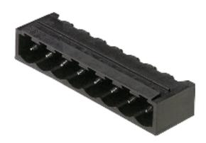
High-temperature-resistant male connector, packed in box or tape. In tape with 1.5 mm solder pin optimised for automatic assembly. 3.2 mm solder pin suitable for reflow and wave soldering. These male connectors can be labelled and coded.
