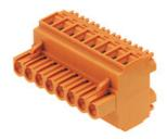
Female connectors with two clamping yoke screw connections per pole for conductor connection with 90° & Damp; 270° outlet direction. The female connectors provide space for labelling and can be coded. Packed in cardboard box.
