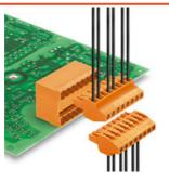
Socket connectors with clamping yoke screw connection for conductor connection with a right-angle (90° or 270°) outlet direction. The female connectors provide space for labelling and can be coded. Can be fastened with flange or release latch. They feature an integrated plus/minus screw, protection against false insertion under clamping yoke. They are delivered with an opened clamping yoke. • 0.2-2.5 mm2 (IEC) / 26-12 AWG (UL)
