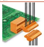
Socket connectors with clamping yoke screw connection for conductor connection with a right-angle (90° or 270°) outlet direction. The female connectors provide space for labelling and can be coded. Can be fastened with flange or release latch. They feature an integrated plus/minus screw, protection against false insertion under clamping yoke. They are delivered with an opened clamping yoke.
