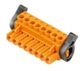
Socket connectors with clamping yoke screw connection for conductor connection with 270° outlet direction and release lever or release latch mechanism. The female connectors provide space for labelling and can be coded. Packed in cardboard box.br/>
