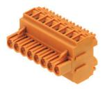
Female connectors with two clamping yoke screw connections per pole for conductor connection with 90° & pole for conductor connection with 90° & pole for labelling and can be coded. Packed in cardboard box.
