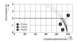
Derating curve for: PTPM 0.2/..-P-2.5 with PTSM 0.5/..-HH-2.5-THR R..
