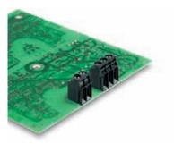
Through Hole Reflow (THR), high-temperature-resistant PCB terminal with proven clamping yoke connection at 5.08 mm pitch, conductor outlet direction 90°, suitable for conductor cross-sections up to 6.0 mm².
