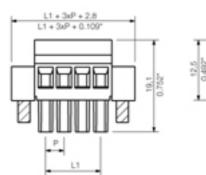
Clamping yoke connection
